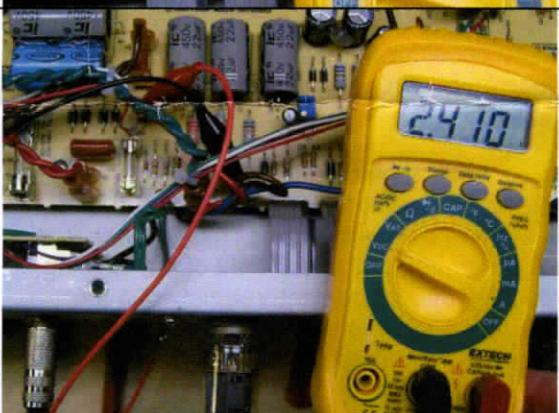
To adjust the bias: Put a jumper clip on the red transformer lead (P2) and another on the brown (P3). Plug in speaker, insert tubes, warm up amp, turn master volume off. Adjust the trimpot until you get a reading of 2.4 to 2.7 volts across these two leads. **Remember that the actual voltages are over 330V and you're only measuring the difference between them!**
